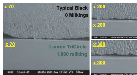
Fig. A Side-by-side comparison results between Lauren Liners and Typical Black Organic Liners.
